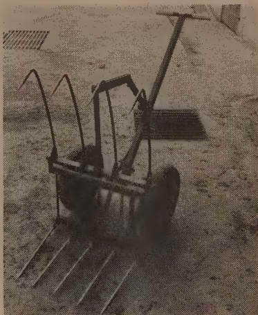
This silage dolly on a dairy in southern Germany represents the intermediate scale between a silage fork and a front-end loader. Push the dolly into the pile, raise the handle to close the jaws, and wheel it away to your livestock.
